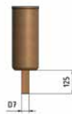
Fixed Copper Conductor FC Fig. 21
